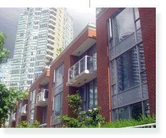
Masonry veneer consists of a single layer (wythe) of masonry units (typically clay brick) and mortar. Masonry is a very durable cladding with maintenance and renewal activities focused on cleaning and occasional repointing (renewal of mortar joints).
